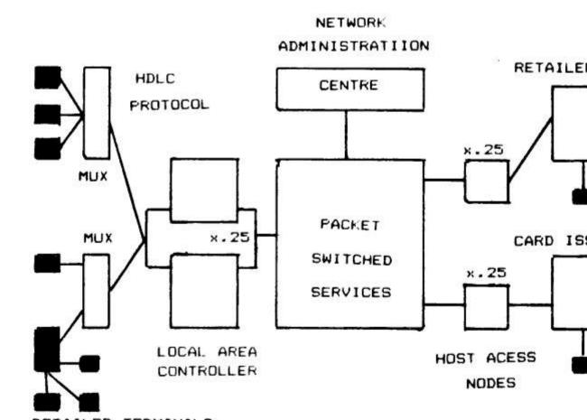
Electronic funds transfer involves the use of point-of-sale terminals at stores and other retail outlets. This system enables automatic debit and credit transfers for purchases by customers with a debit or credit card. The POS terminals connect over the public switched telephone network and/or the packet switched network with both the retailer's bank and the card issuing organisation so that all accounting action involved in a transaction is completed at the time of purchase. (Figure 5).
